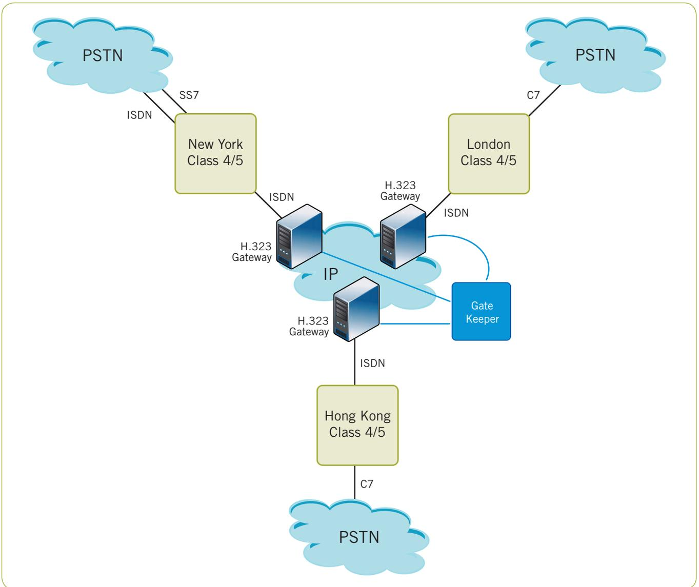
Figure 2. VoIP Enabled with Discrete VoIP Gateways
