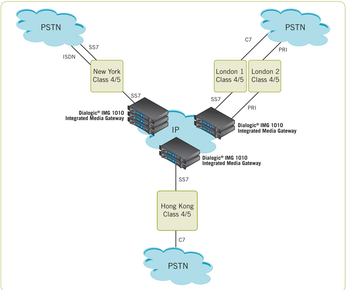
Figure 3. Dialogic® IMG 1010 Integrated Media Gateway Integrated with VoIP Distributed Components
